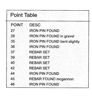
Note: All Rebars Set are 5/8" Epoxy Coated 30" Long Capped with McGannon Surveying LLC 7154 as standard and required by the State of Ohio.
