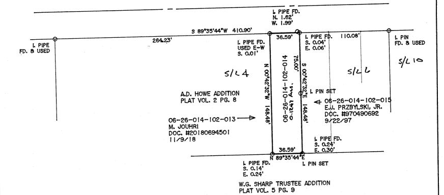
DIMENSIONS SHOWN ON THIS PLAT ARE EXPRESSED IN FEET AND DECIMAL PARTS THEREOF, ALL BEARINGS ARE TO AN ASSUMED MERIDIAN AND ARE USED TO INDICATE ANGLES ONLY. PERMANENT MONUMENTS WERE FOUND OR SET AT ALL POINTS INDICATED HEREON, ALL OF WHICH I GERTIFY TO
