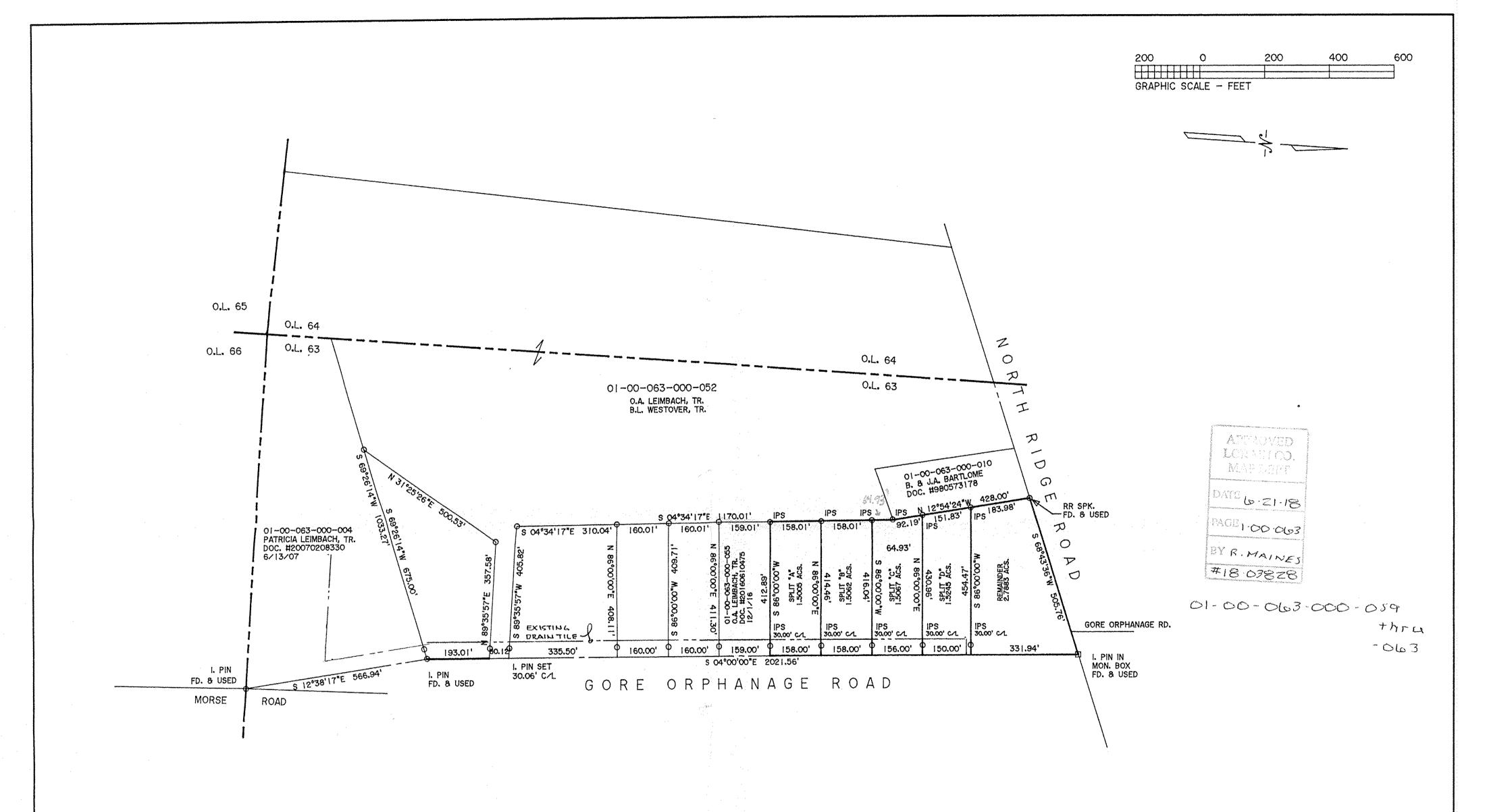
DIMENSIONS SHOWN ON THIS PLAT ARE EXPRESSED IN FEET AND DECIMAL PARTS THEREOF, ALL BEARINGS ARE TO AN ASSUMED MERIDIAN AND ARE USED TO INDICATE ANGLES ONLY. PERMANENT MONUMENTS WERE FOUND OR SET AT ALL POINTS INDICATED HEREON, ALL OF WHICH I CERTIFY TO BE CORRECT.
