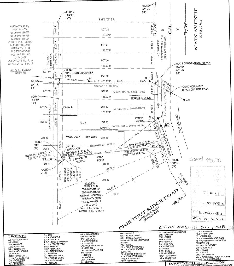
SIZE OF MONUMENTATION FOUND IS NOTED ON MAP AND IS AT GRADE UNLESS NOTED OTHERWISE. MONUMENTATION ABOVE GRADE IS NOTED (+) AND BELOW GRADE IS NOTED (-). THE SIZE OF MONUMENTATION I.D. IS NOTED WHERE EXISTS AND LEGIBLE. IRON RODS SET ARE 30" LONG, 5½" DIAMETER REBAR WITH I.D. CAP "HAYWOOD 8284" AND SET TO GRADE. SURVEYOR WALLS SET INCLUDE I.D. DISK. CORNERS NOT MONUMENTED ARE LABELED CALCULATED POINT.
