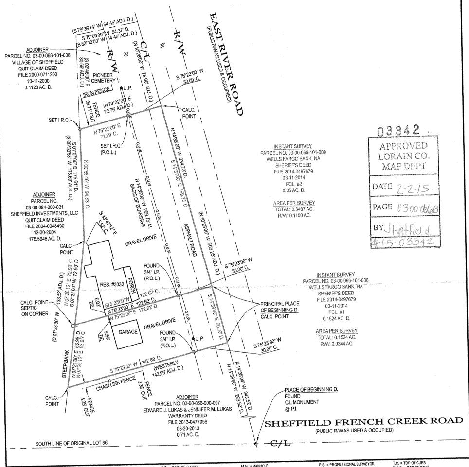
LEGEND: A/C = AIR CONDITIONER AC. ≈ ACRE ADJ. = ADJOINER ADJC. = ADJACENT B.L. = BUILDING LINE B.O.C. = BACK OF CURB CH. = CHORD CONC. = CONCRETE C., CALC. = CALCULATED C.B. = CATCH BASIN C.O. = CLEAN OUT C/L = CENTERLINE D.S. = DOWNSPOUT D.H. = DRILL HOLE E.O.P. = EDGE OF PAVEMENT E.O.W. = EDGE OF WATER ELEC. = ELECTRIC ELEV. = ELEVATION E.M. = ELECTRIC METER EX. = EXISTING F.F. = FINISHED FLOOR F.G. = FINISHED GRADE F.H. = FIRE HYDRANT
