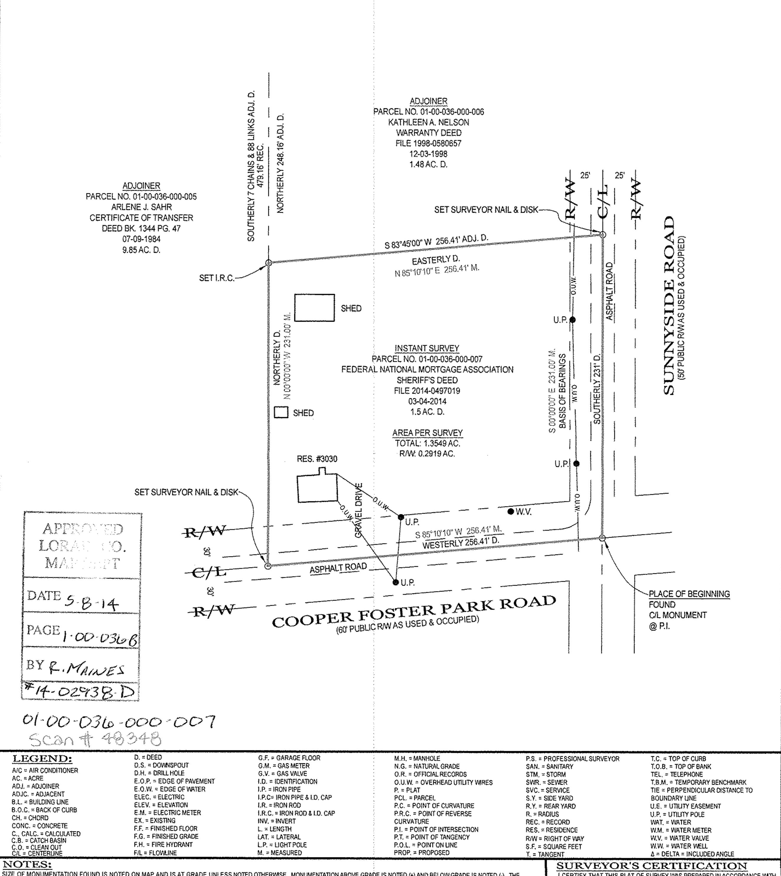
SIZE OF MONUMENTATION FOUND IS NOTED ON MAP AND IS AT GRADE UNLESS NOTED OTHERWISE. MONUMENTATION ABOVE GRADE IS NOTED (+) AND BELOW GRADE IS NOTED (-). THE MONUMENTATION I.D. IS NOTED WHERE EXISTS AND LEGIBLE. IRON RODS SET ARE 30" LONG, 5/8" DIAMETER REBAR WITH I.D. CAP "HAYWOOD 8284" AND SET TO GRADE, SURVEYOR NAILS SET INCLUDE I.D. DISK. CORNERS NOT MONUMENTED ARE LABELED CALCULATED POINT.
