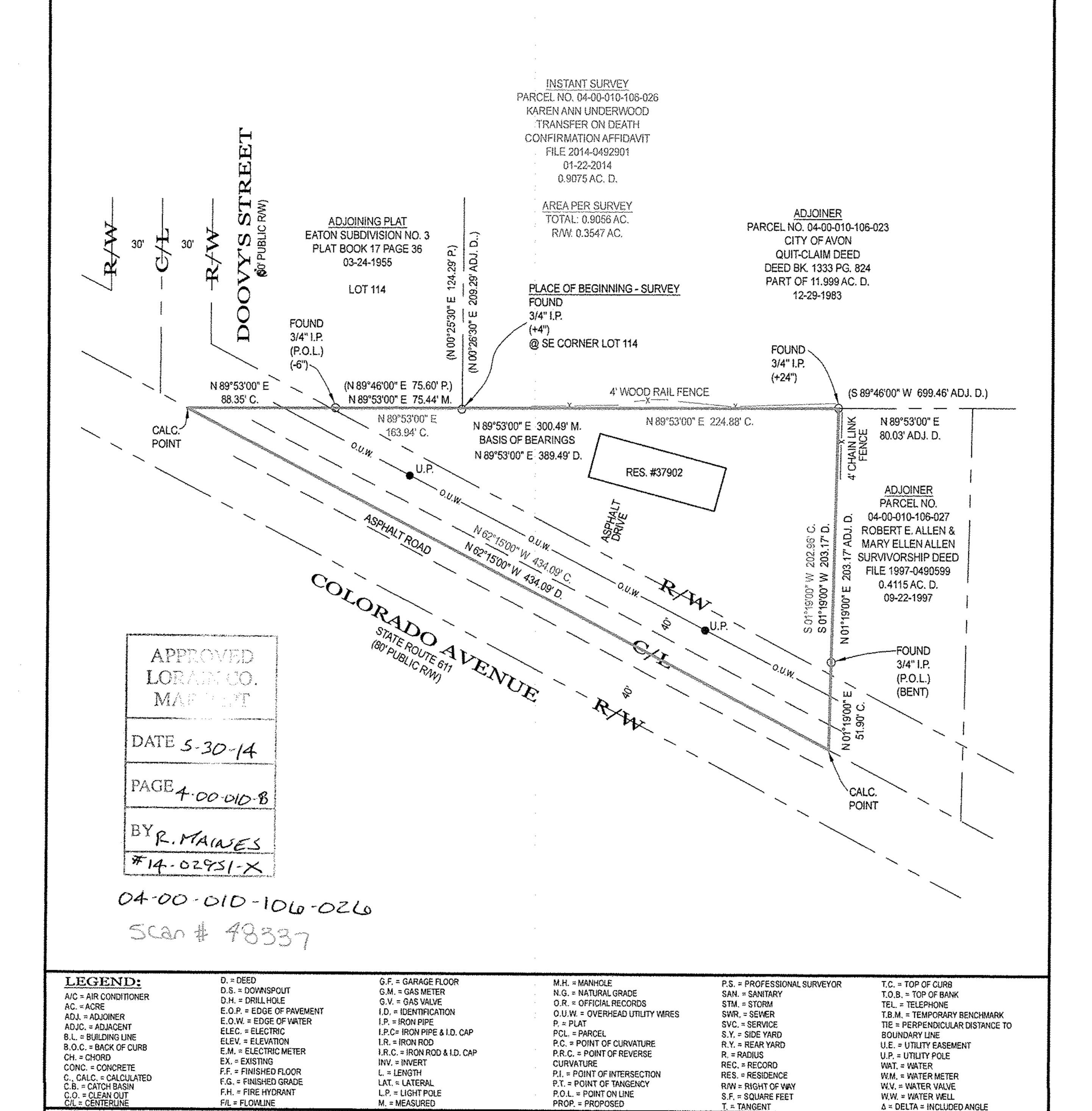
NOTES: SIZE OF MONUMENTATION FOUND IS NOTED ON MAP AND IS AT GRADE UNLESS NOTED OTHERWISE, MONUMENTATION ABOVE GRADE IS NOTED (+) AND BELOW GRADE IS NOTED (-). THE MONUMENTATION I.D. IS NOTED WHERE EXISTS AND LEGIBLE. IRON RODS SET ARE 30" LONG, 5/8" DIAMETER REBAR WITH I.D. CAP "HAYWOOD 8284" AND SET TO GRADE, SURVEYOR NAILS SET INCLUDE I.D. DISK. CORNERS NOT MONUMENTED ARE LABELED CALCULATED POINT.
