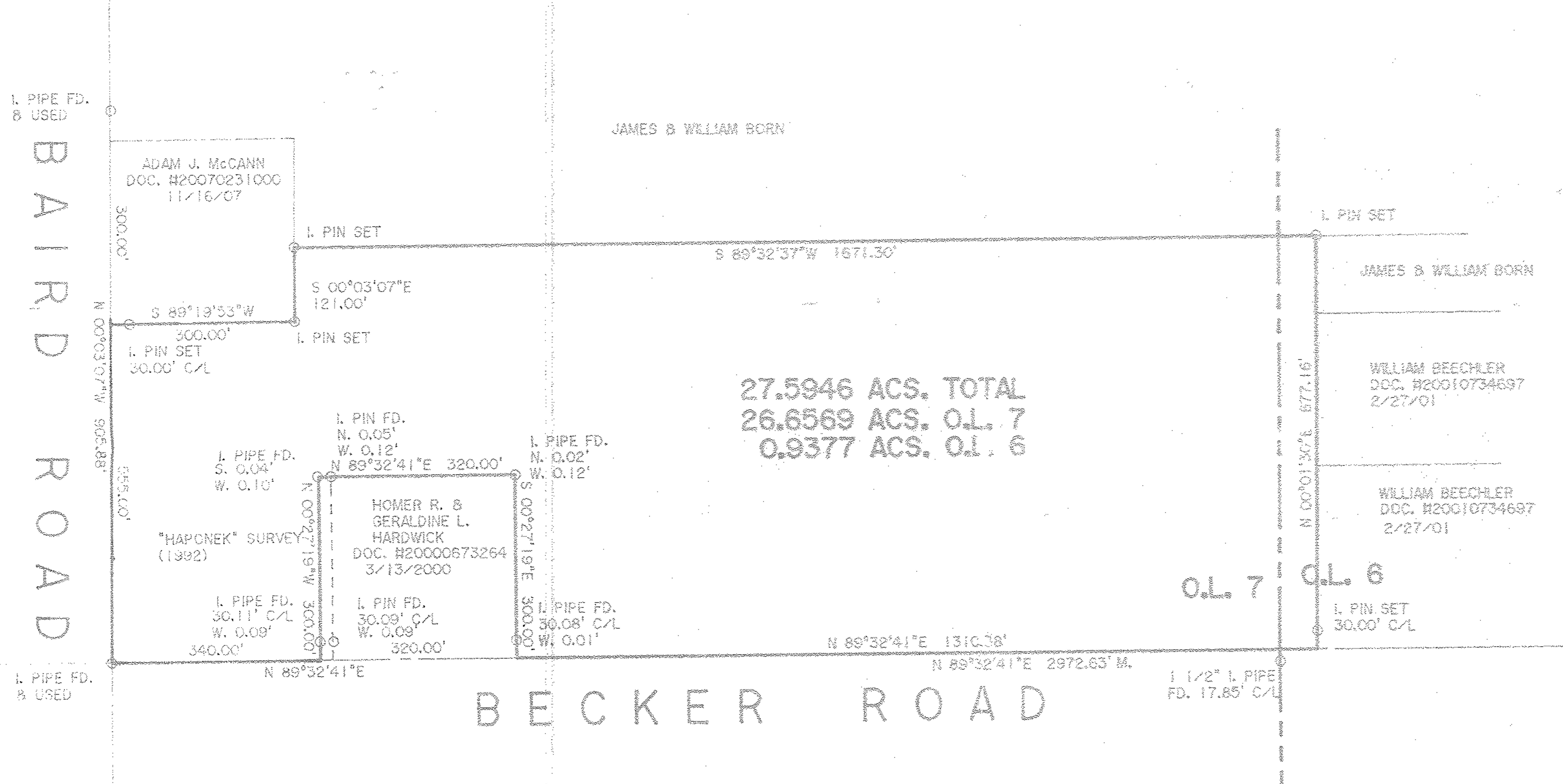
DIMENSIONS SHOWN ON THIS PLAT ARE EXPRESSED IN FEET AND DECIMAL PARTS THEREOF. ALL BEARINGS ARE TO AN ASSUMED MERIDIAN AND ARE USED TO INDICATE ANGLES ONLY. PERMANENT MONUMENTS WERE FOUND OR SET AT ALL POINTS INDICATED HEREON, ALL OF WHICH I CERTIFY TO BE CORRECT.
