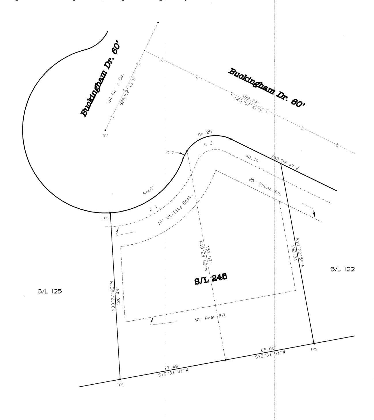
C1 L= 69.77' CA=66 deg 37' 29" C= 65.90' N 53 deg 13' 47"E C2 L= 6.06' CA= 13 deg 53' 29" C= 6.05' N 26 deg 51' 47"E C3 L= 35.88'' CA= 82 deg 13' 41" C= 32.88' N 74 deg 55' 22"E
