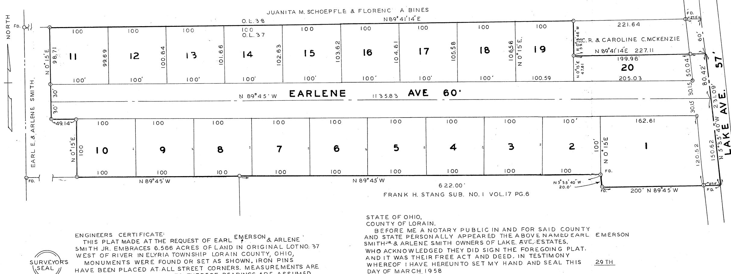
HAVE BEEN PLACED AT ALL STREET CORNERS. MEASUREMENTS ARE IN FEET AND DECIMAL PARTS THEREOF. BEARINGS ARE ASSUMED AND ARE FOR DESCRIBING ANGLES ONLY ALLOF WHICH I CERTIFY TO BE CORRECT -O-INDICATES IRON PINS FOUND OR SET. RAY E. HOLLIS. CIVIL ENGINEER & SURVEYOR
