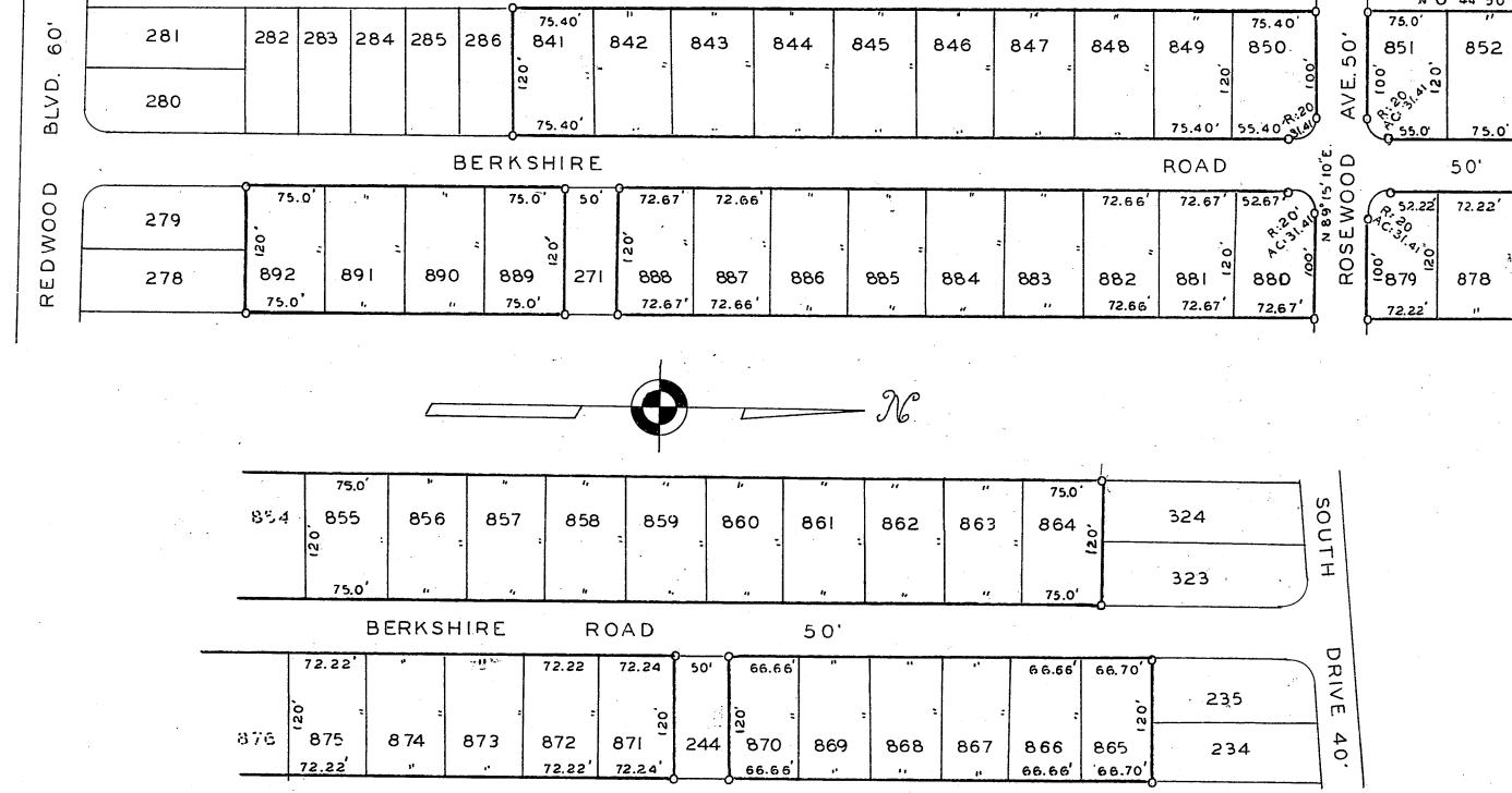
THIS PLAT MADE AT THE REQUEST OF YODER, INC. EMBRACES 10.479 A CRES OF LAND IN SECTION 18 AVON TOWNSHIP NOW AVON LAKE VILLAGE, LORAIN COUNTY, OHIO, IRON PINS WERE FOUND OR SET AS SHOWN, MEASUREMENTS ARE INFEET AND DECIMAL PARTS THEREOF BEARINGS USED ARE ASSUMED AND ARE FOR THE PURPOSE OF DESCRIBING ANGLES ONLY. ENGINEER ALL OF WHICH I CERTIFY TO BE CORRECT
