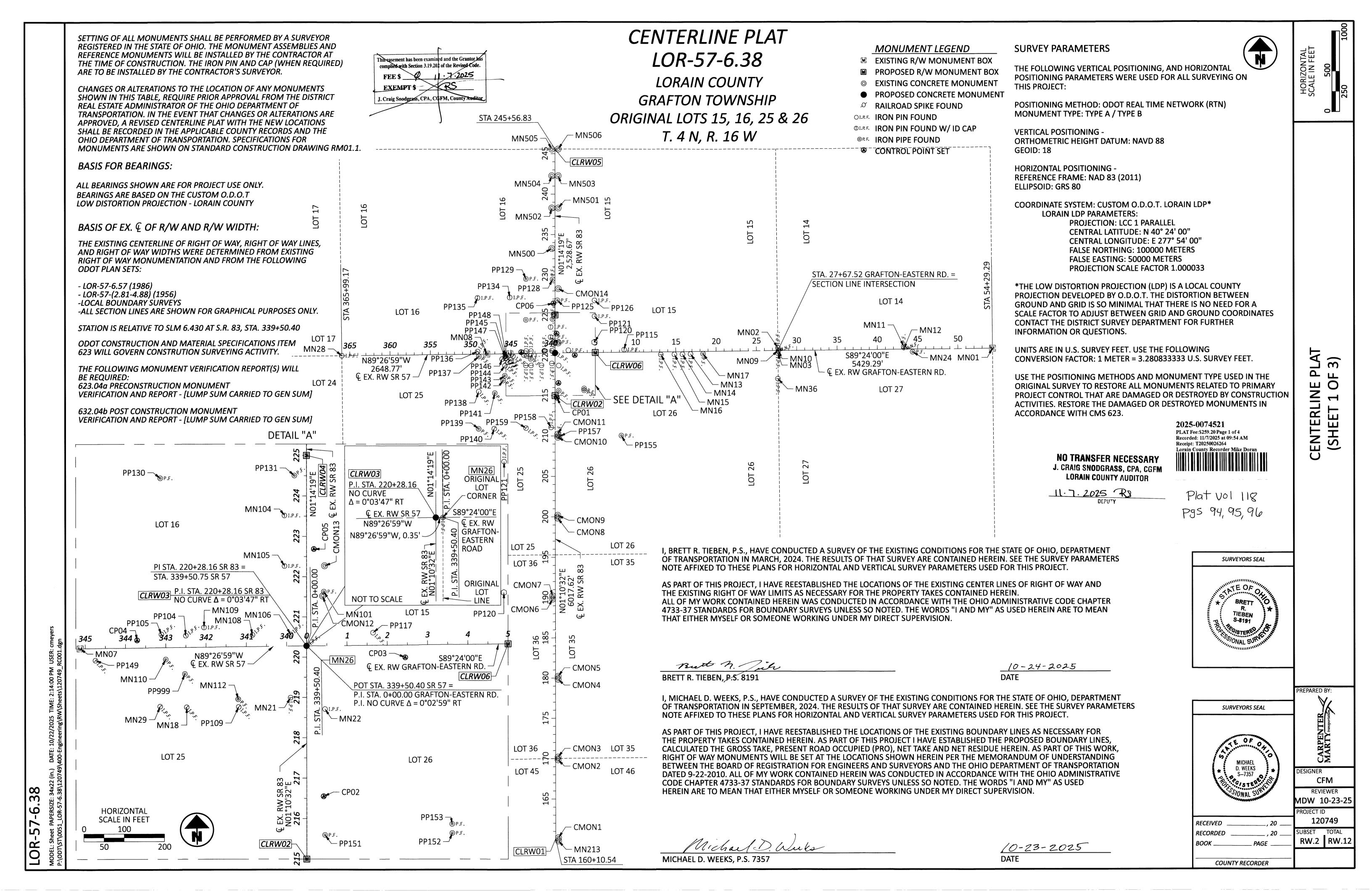
\*THE LOW DISTORTION PROJECTION (LDP) IS A LOCAL COUNTY PROJECTION DEVELOPED BY O.D.O.T. THE DISTORTION BETWEEN GROUND AND GRID IS SO MINIMAL THAT THERE IS NO NEED FOR A SCALE FACTOR TO ADJUST BETWEEN GRID AND GROUND COORDINATES CONTACT THE DISTRICT SURVEY DEPARTMENT FOR FURTHER INFORMATION OR QUESTIONS.
