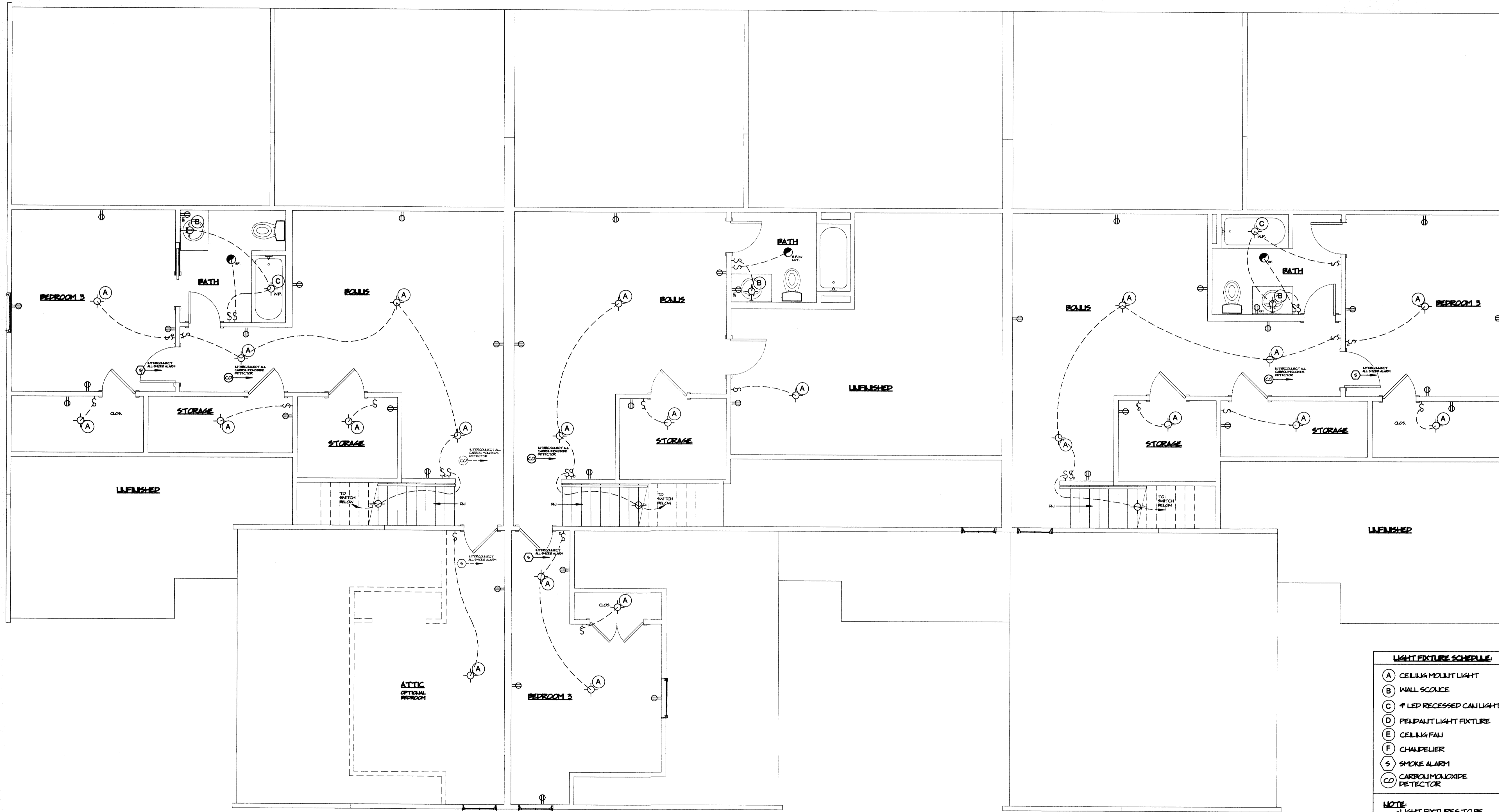
SECOND FLOOR POWER/LIGHTING PLAN 1/4" = 1'-0"
