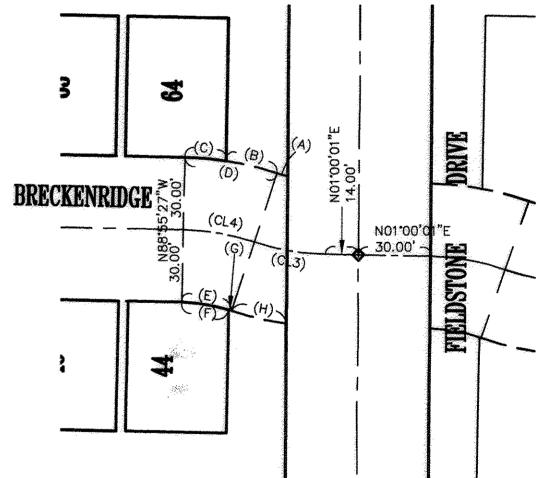
ALL SUBLOTS SHOWN HEREON SHALL HAVE THE FOLLOWING BEARINGS: NORTH & SOUTH DIRECTION = N.01°04'33"E. EAST & WEST DIRECTION = N.88'55'27"W.
