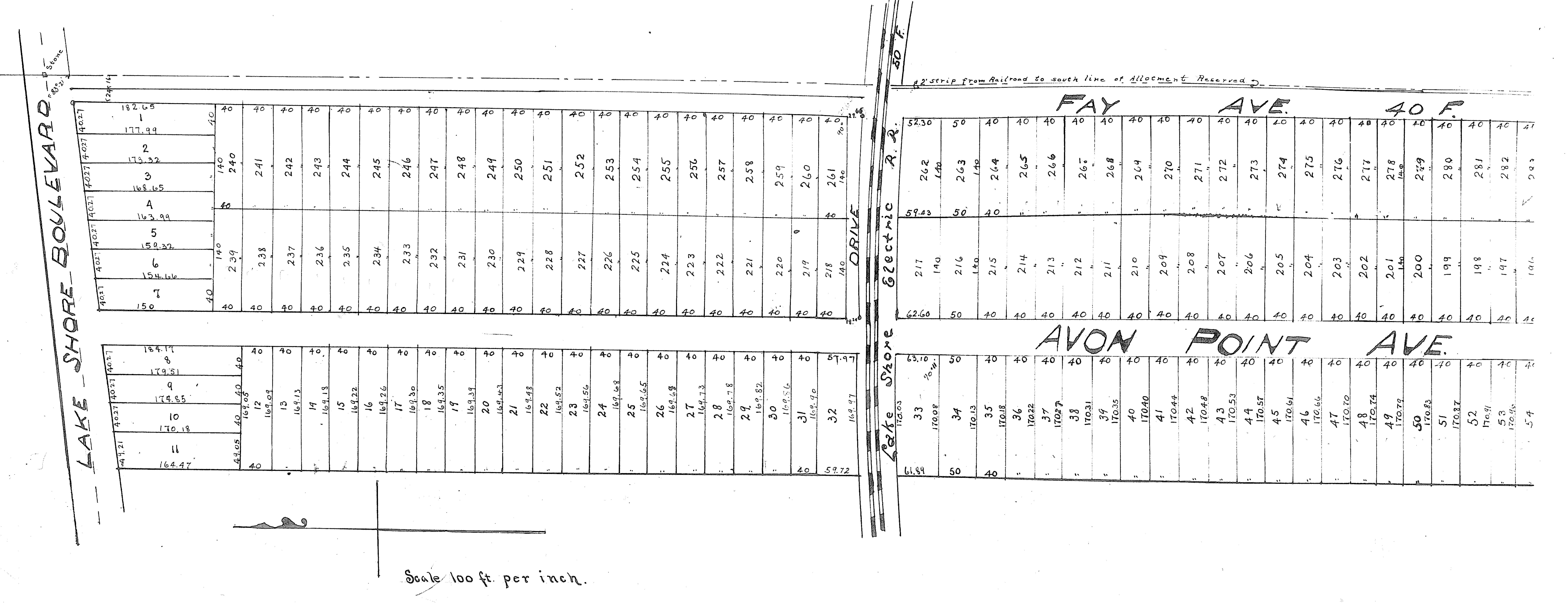
Stone monuments are located at all points so indicated on the plat. Distances are given in fect and decimal parts thereof. Scale 100 ft. per inch.
